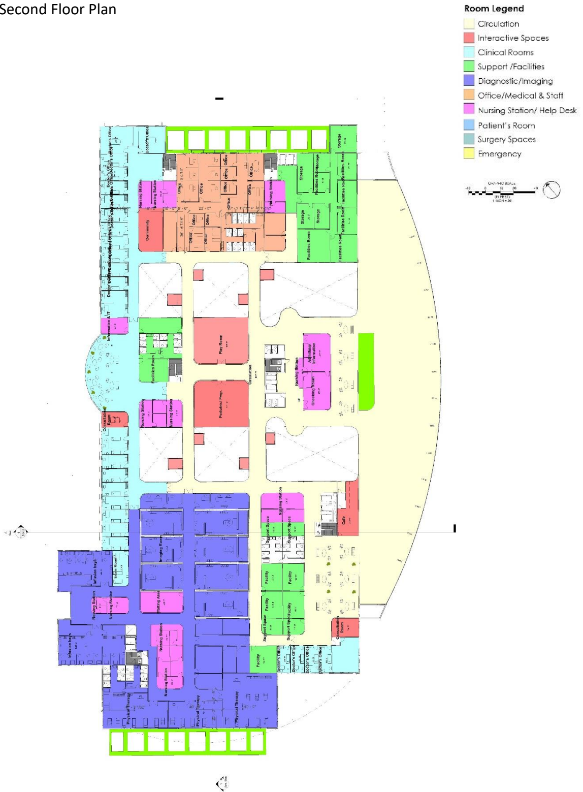
Figure 69. Second Floor Level (Image credit by author)
